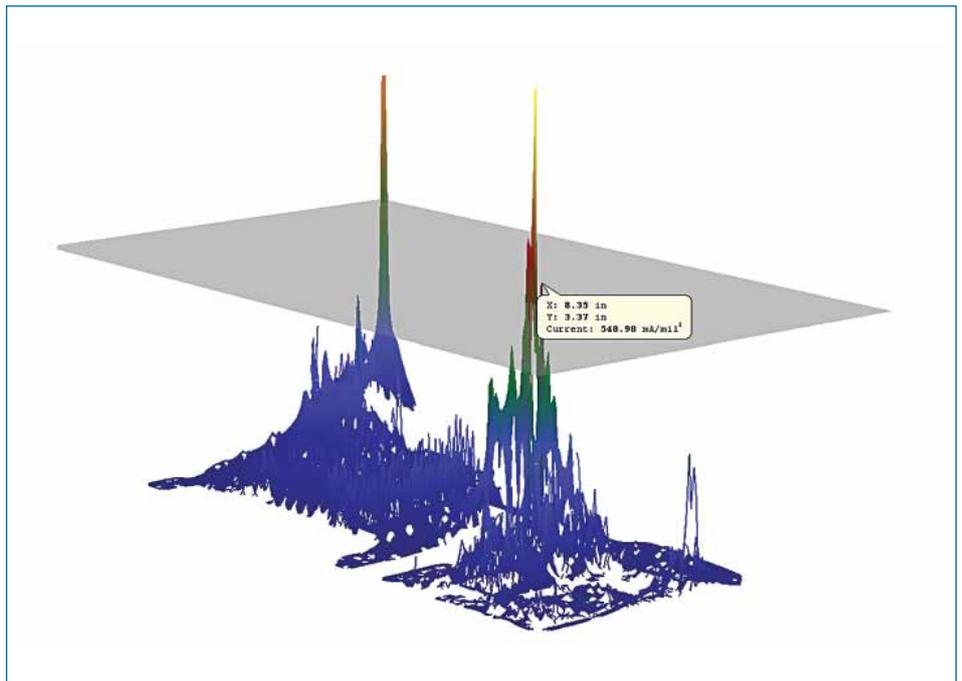
Fig. 4: Three-dimensional plot of current density on a power plane, the results of analysis performed with HyperLynx power integrity.
