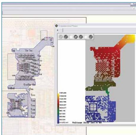
Fig. 3: Plot of DC voltage, the results of a power plane analysis.
