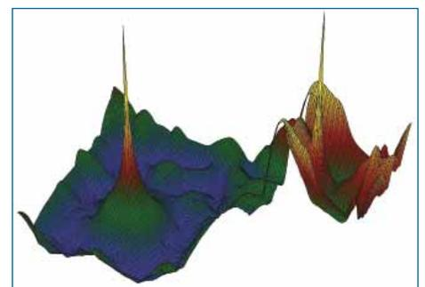
Fig. 2: Results of a pre-route noise analysis of a power distribution network in HyperLynx power integrity.
